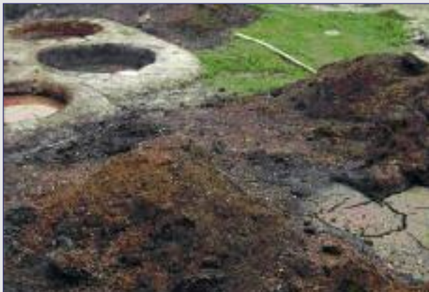
3) Deliming/pickling: using a slurry of dried and ground pomegranate skins (1-2 weeks depending on the thickness). The fruit acids provide a natural and gentle neutralisation of the lime and a gentle pickling to the extent of starting a vegetable tannage. The exhaust material is piled and dried after use, providing winter fuel for heating.
