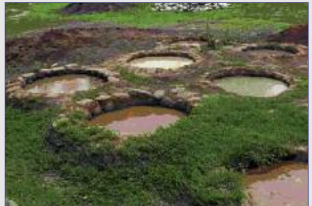
4) Tannage: done in a vat, using a dried, ground root from a plant related closely to rhubarb (genus rheum). Up to 10 kg per pelt is required to complete the tannage.
