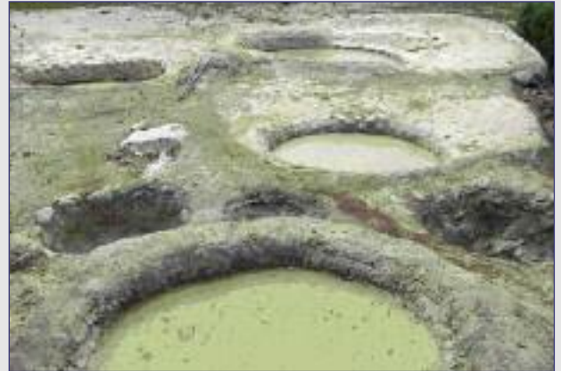
2) Liming: in stone vats, for between 1 – 3 weeks, depending on the raw material (sheep, goat or bovine) and, of course, the intended end use.
