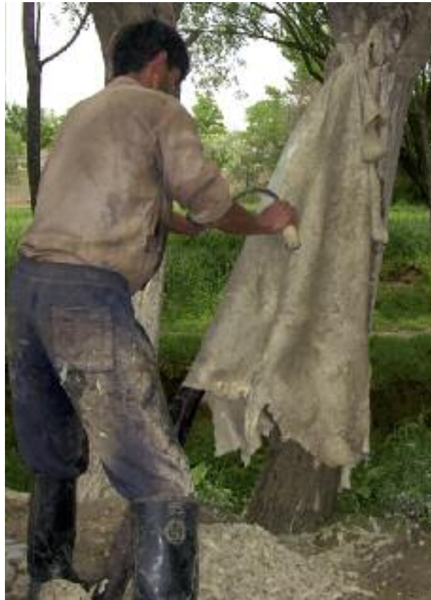
Fleshing after liming — done by hand, over a log leant up against a tree. A long and arduous task, requiring great hand-eye coordination to avoid damaging the pelt.
